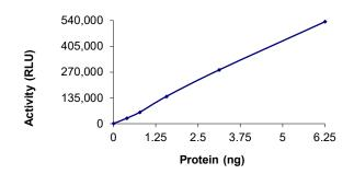
The specific activity of GSK3β was determined to be **224 nmol** /min/mg as per activity assay protocol, and was equivalent to **201 nmol/min/mg** as per radiometric assay.
