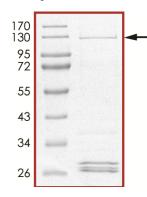
The purity of PDE6B was determined to be >90% by densitometry.
