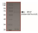
The purity of BRAF (R506\_K507 insVLR) protein was determined to be >70% by densitometry, approx. MW 69 kDa.
