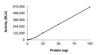
The specific activity of ALK (I1171N D1203N) was determined to be **19 nmol/min/mg** as per activity assay protocol.
