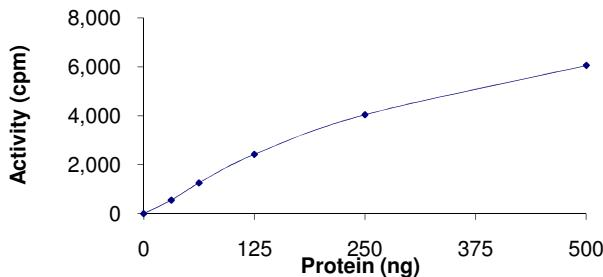
The specific activity of FASTK was determined to be **1.0 nmol/min/mg** as per activity assay protocol.
