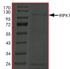
The purity of RIPK1 was determined to be **>70%** by densitometry, approx. MW **108 kDa**.
